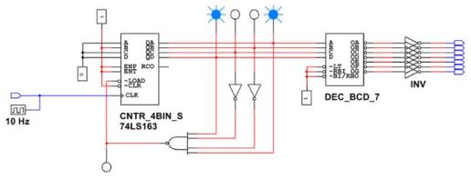
Using the CDS, enter the 2 to 9 Binary Up Counter in PLD Mode. By monitoring the logic probes attached to outputs QD, QC, QB, and QA, verify that the circuit is working as expected (Is the count 2 to 9?). If the
