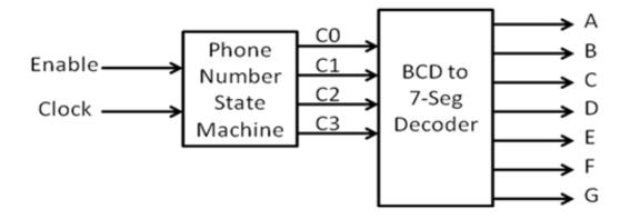
In addition to the clock input required for all state machines, this design's second input is Enable (EN). Whenever the EN input is a logic (1), the outputs will continuously cycle through the four digits of the phone number. Whenever the EN input is a logic (0), the outputs will hold at their current values.
