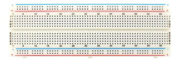
Note how all holes in the selected row are connected together, so the holes in the selected column. The set of connected holes can be called a node:
