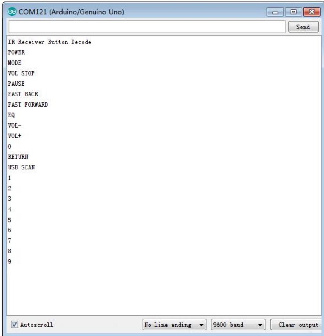
**Then, the remote control is aligned with the IR receiver and the corresponding numbers and symbols are displayed on the monitor**
